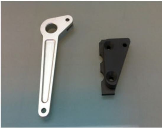
<--- Both these parts are examples of undyed, "clear" anodizing, the only difference is the thickness of the anodizing!
